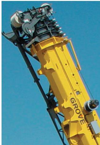
The superstructure features a full power five section MEGAFORM boom that can reach to a maximum tip height of 150 ft. The TWIN-LOCK boom pinning system provides pre-selection of boom extension modes to efficiently pin boom sections automatically.
